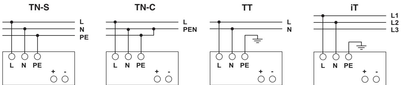
The 100 V AC ... 240 V AC connection is made using the L and N screw connections.
